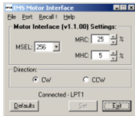
The IMS Motor Interface GUI (Graphical User Interface) simplifies use with single screen interface for configuring the MDrive.
